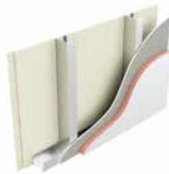
Type LE2: Two layers of plasterboard, stud, sheathing board, 50mm K15 Insulation
