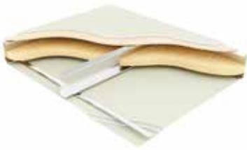
Type F4: Three layers of plasterboard, resilient bars, joists with mineral wool between, 15mm plywood, 19mm British Gypsum Plank
