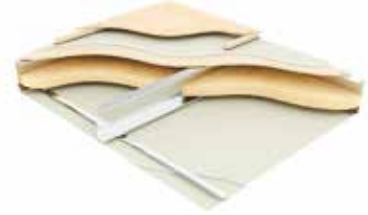
Type F3: Two layers of plasterboard, resilient bars, joists with mineral wool between, 15mm plywood, 19mm British Gypsum Plank, 53mm Danskin acoustic battens, 18mm V313 chipboard
