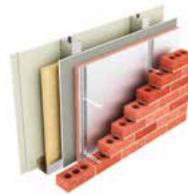
Type EC1i: Two layers of plasterboard, stud with mineral wool between, sheathing board, insulation, cavity, brickwork
