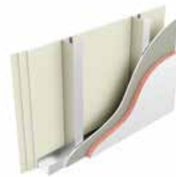
Type LE6: Three layers of plasterboard, stud, sheathing board, 50mm K15 Insulation
