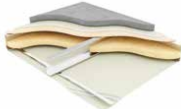
Type F10: Three layers of plasterboard, resilient bars, joists with mineral wool between, 15mm plywood, 19mm British Gypsum Plank, Collecta Screedboard 28
