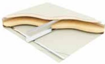
Type F1: Two layers of plasterboard, resilient bars, joists with mineral wool between, 15mm plywood, 19mm British Gypsum Plank
