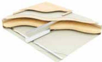
Type F7: Two layers of plasterboard, resilient bars, joists with mineral wool between, 15mm plywood, 19mm British Gypsum Plank, 70mm Collecta Deckfon acoustic battens, 18mm V313 chipboard
