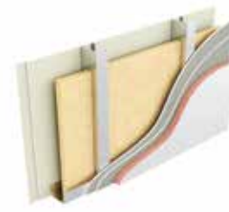
Type E3i: Two layers of plasterboard, stud with mineral wool between, two layers of sheathing board, 50mm K15 Insulation
