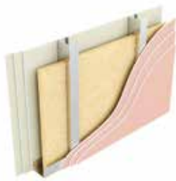
Type L6: Three layers of plasterboard, stud with mineral wool between, three layers of plasterboard
