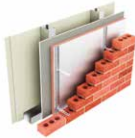
Type EC1: Two layers of plasterboard, stud, sheathing board, insulation, cavity, brickwork
