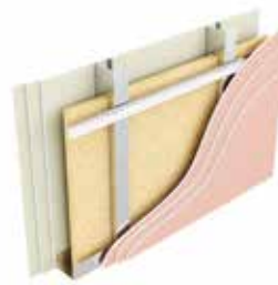
Type L7: Three layers of plasterboard, stud with mineral wool between, resilient bar, three layers of plasterboard
