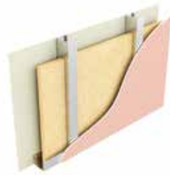
Type H1i: Layer of plasterboard, stud with mineral wool between, layer of plasterboard
