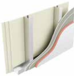
Type LE7: Three layers of plasterboard, stud, two layers of sheathing board, 50mm K15 Insulation
