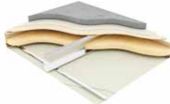
Type F8: Two layers of plasterboard, resilient bars, joists with mineral wool between, 15mm plywood, 19mm British Gypsum Plank, Collecta Screedboard 28
