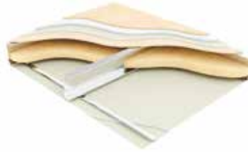
Type F2: Two layers of plasterboard, resilient bars, joists with mineral wool between, 15mm plywood, 19mm British Gypsum Plank, 8mm Cloud 9 Underlay, 12mm OSB
