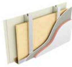
Type E2i: Two layers of plasterboard, stud with mineral wool between, sheathing board, 50mm K15 Insulation
