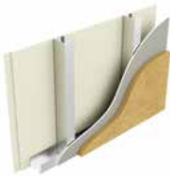
Type LE4: Two layers of plasterboard, stud, sheathing board, 75mm Rockwool Duoslab Insulation
