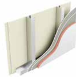
Type LE3: Two layers of plasterboard, stud, two layers of sheathing board, 50mm K15 Insulation
