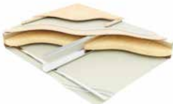
Type F9: Three layers of plasterboard, resilient bars, joists with mineral wool between, 15mm plywood, 19mm British Gypsum Plank, 70mm Collecta Deckfon acoustic battens, 18mm V313 chipboard
