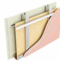
Type H4i: Two layers of plasterboard, resilient bar, stud with mineral wool between, resilient bar, two layers of plasterboard
