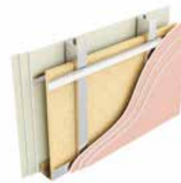
Type L8: Three layers of plasterboard, resilient bar, stud with mineral wool between, resilient bar, three layers of plasterboard
