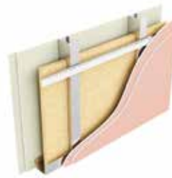
Type H3i: Two layers of plasterboard, stud with mineral wool between, resilient bar, two layers of plasterboard
