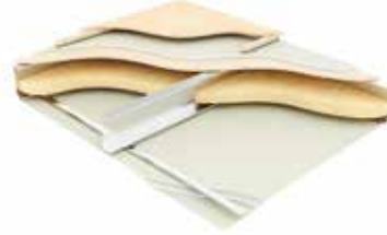
Type F6: Three layers of plasterboard, resilient bars, joists with mineral wool between, 15mm plywood, 19mm British Gypsum Plank, 53mm Dansk acoustic battens, 18mm V313 chipboard
