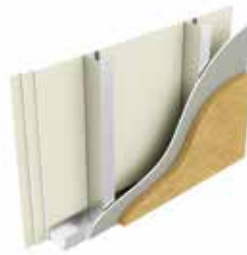
Type LE8: Three layers of plasterboard, stud, sheathing board, 75mm Rockwool Duoslab Insulation
