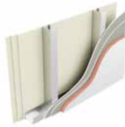
Type LE7: Three layers of plasterboard, stud, two layers of sheathing board, 50mm K15 Insulation
