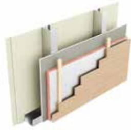
Type EC3: Two layers of plasterboard, stud, sheathing board, insulation, battens, timber cladding
