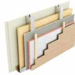
Type EC3i: Two layers of plasterboard, stud with mineral wool between, sheathing board, insulation, battens, timber cladding
